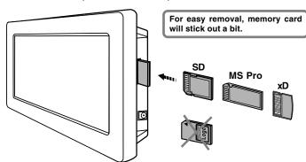
If you cannot easily insert the memory card, you may have inserted it incorrectly. Try to turnover the card and then insert again
